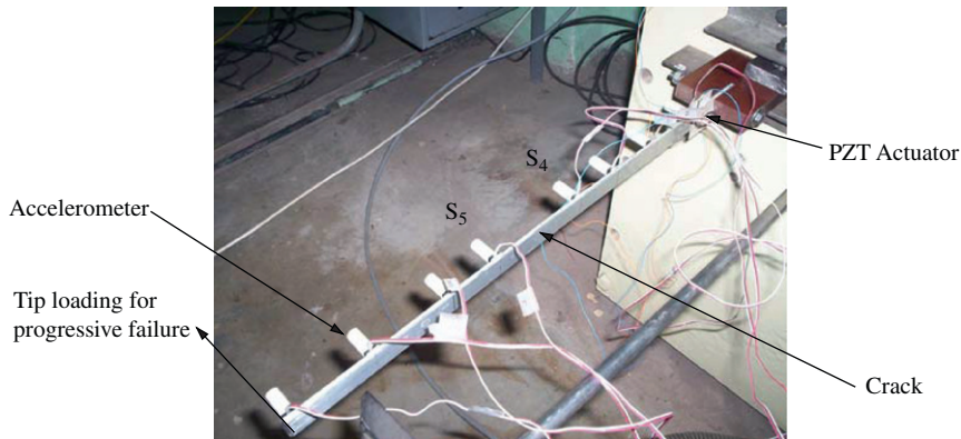
Fig. 9. Instrumented sample with eight-sensor configuration.
